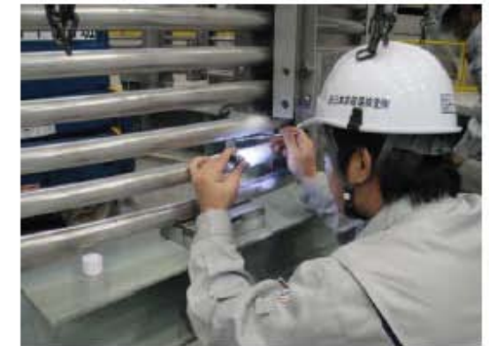
Global He Leak Test & Dye Penetrant Test
