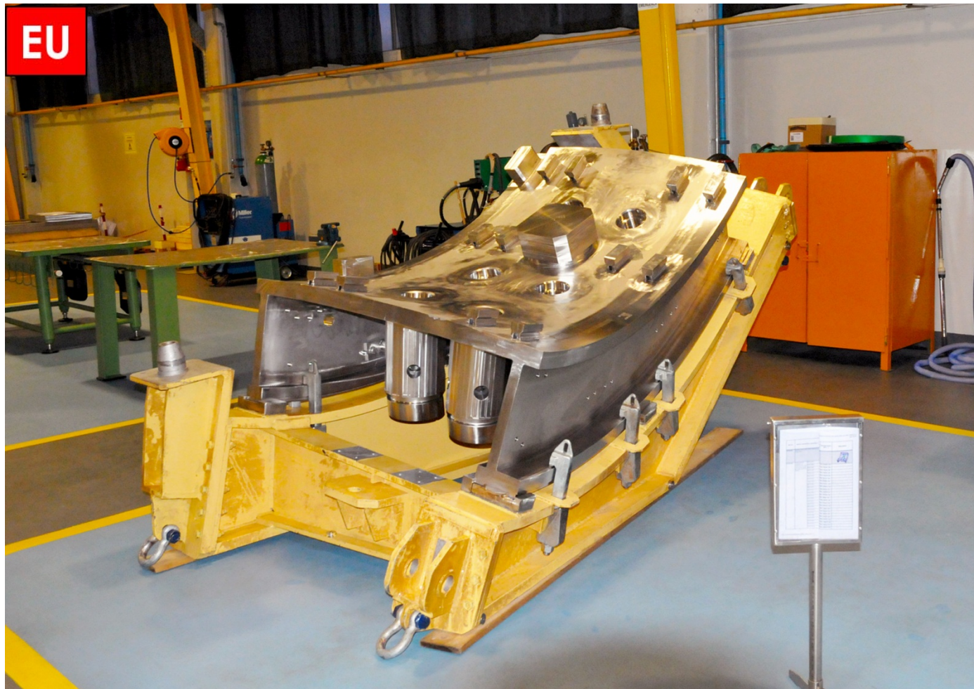
Mock-up of the inboard part of a vacuum vessel segment, produced by Walter Tosto SpA, in Chieti, Italy.
